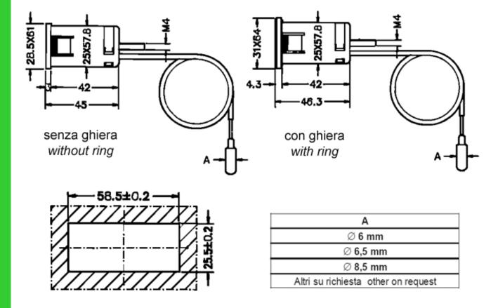
Case: shockproof ABS, standard colours black or white, other colours on request. Fixing system: moulded-in elastic tabs, metallic bracket on request (TR 58.25.42 PS).
